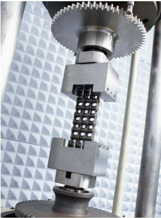
Fatigue strength determined with a high-frequency pulser
