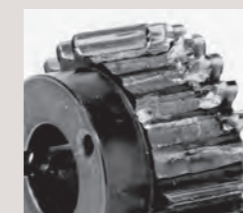
Example of failure due to insufficient bending strength
