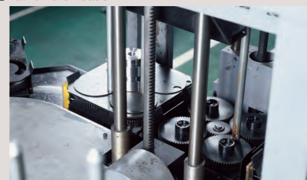
SRO Round Rack used as a workpiece storage device (lifting/lowering table)
