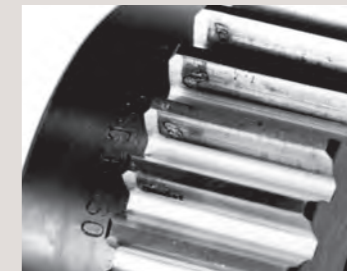
Poor tooth contact and pitting
