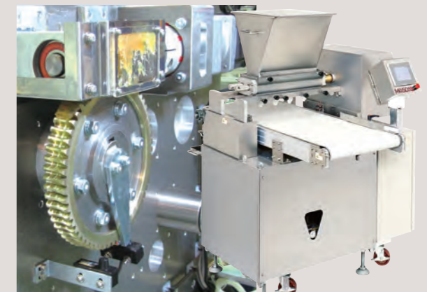
KWGDL Duplex Worm Wheels and AGDL Worm Wheels used for indexing and driving, for accurate filling of a fixed amount of ingredients
