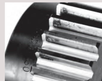
Poor tooth contact and pitting
